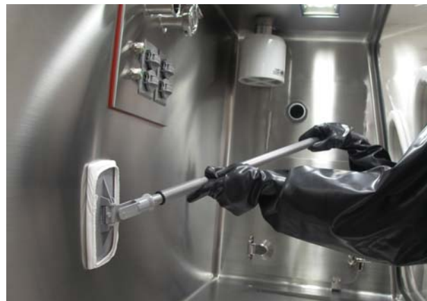
Figure 1. Isolator cleaning tool in use
