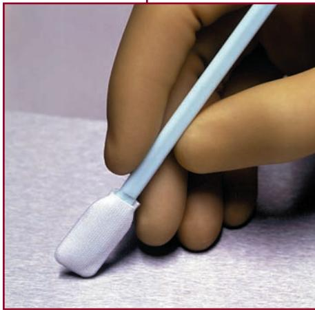
*Figure 1 – A polyester knit swab used for surface sampling*
