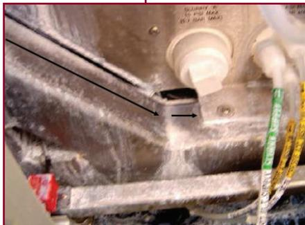
*Figure 2 – Black arrows show surfaces after a single cleaning. Some slurry removed, but multiple applications will be required to remove all the residue. Picture is somewhat out of focus.*
