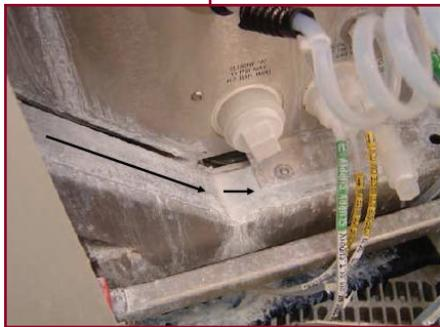
*Figure 1 – Lower corner of CMP tool before cleaning. Black arrows show area to be cleaned.*
