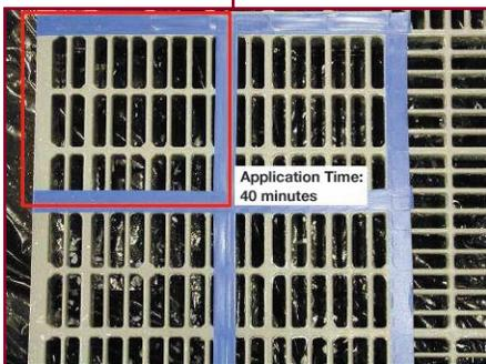
*Figure 4 – Floor grate after a single cleaning. Most of the residue was removed but some additional cleaning is required. Material under floor grate is a black plastic bag.*
