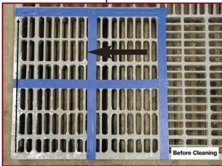
*Figure 3 – Floor grate before cleaning. Black arrow indicates the surface that will show the most dramatic results in Figure 4.*
