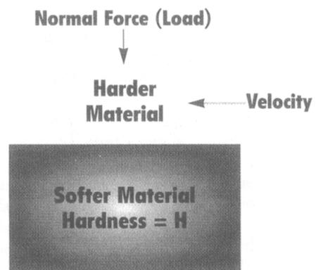
*Figure 1. Basic components of a system undergoing abrasion.*
